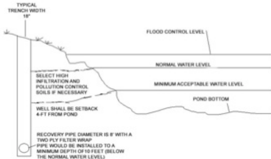
Figure 5.12.2. Schematic for a Typical Stormwater Harvesting Pond
