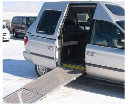
Modifications typically involve cutting and removing the floor structure between the front and rear axles and welding a custom floor constructed from rectangular tubes that is lower by as
