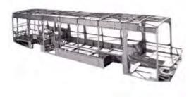
this vehicle type (this issue is discussed further in Chapter 6). Both traditional and stick-built structures are covered with outer panels composed of either stainless steel, aluminum or composite materials.
