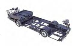
and tires, engine and transmission, fuel system, HVAC, and electrical system. The chassis of a body-on-frame design (10-year buses) are not overhauled but may be repaired during the life of the vehicle. The custom designed chassis are designed to last the full 12-year service life and are overhauled/repaired as necessary. The cost of a typical midlife overhaul of the heavy-duty custom chassis ranges from \$7,000 to \$14,000.
