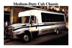
The majority of buses in this category are purpose built using either a front-engine cab chassis or a stripped chassis, both of which are manufactured by medium- and heavy-duty truck manufacturers (e.g., International, Freightliner, and Workhorse). A "final stage" transit vehicle manufacturer (e.g., Champion, Eldorado National, and Goshen Coach) then adds a body and other components to complete construction of the 7-year bus.
